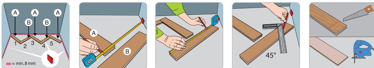
Consider the expansion gap at the sides, when measuring the size of the last plank in the row.
