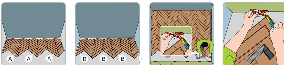
Take a plank and put it in the right direction (groove side towards the end wall). Mark the distance you have measured, and draw a line in a 45° angle. Cut the plank and install it. We advise to use glue on the grooves of very small pieces.
