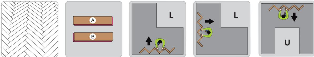
For the herringbone pattern, you need 2 plank types : A-planks and B-planks. When you take a plank and turn the long groove side towards you, the groove continues on the **RIGHT** side for the A-planks and on the **LEFT** side for the B-planks. Always make sure the grooves are pointing towards the laying direction.
