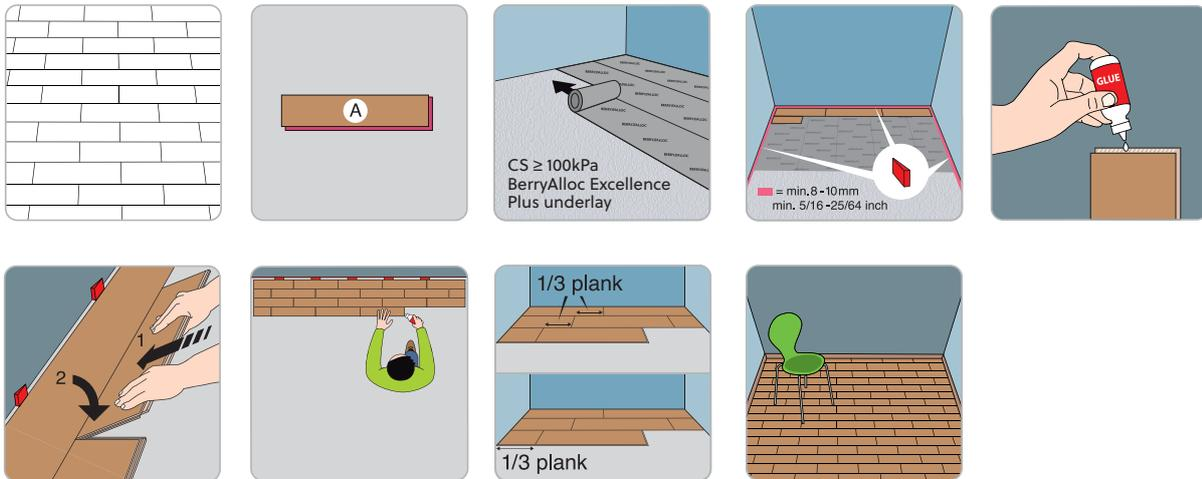
If you choose the shipdeck pattern, you only need the A-planks. Put a first plank in the corner of the room with groove side pointing towards the direction of the installation. Apply glue to the short side of every plank before you install it. Make sure the joints of the planks are staggered 1/3 of their length.
