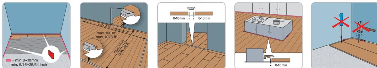
Chateau should be installed as a floating floor which means that the floor should be able to move :
