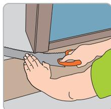
Wooden doorframes should be shortened enough to make a plank and underlay fit underneath. Lay a panel face down next to the doorframe. Saw the panel, then slide the plank under the doorframe. Keep an expansion gap under the doorframe of 8-10mm!
