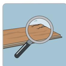
Check all planks for visible defects in optimal light conditions, both before and during installation.
