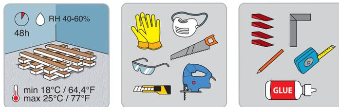
It is important to store the laminate boxes at room temperature for at least 48 hours before the installation. Do not open the packs and stack them in a way so they have maximum contact with the air. The floor should be installed at a room temperature of 18-25°C and a relative humidity of 40-60%.
