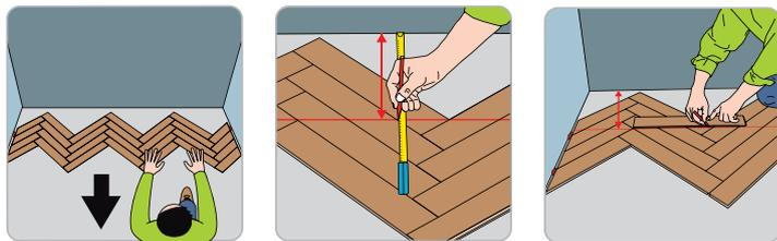
Shift the installed floor towards the starting wall and draw a straight cutting line across the whole row, parallel to the wall.
