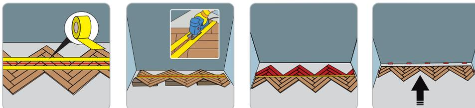
Continue with the installation row per row : a series of A-planks, and then a series of B-planks.
